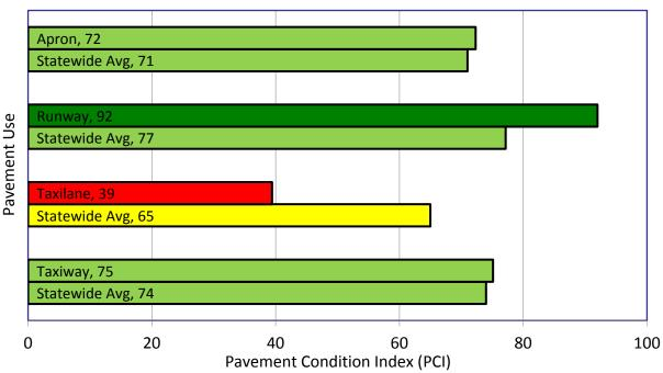
Figure 6. Area-weighted PCI by pavement use.
