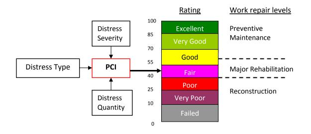
Figure 3. PCI rating scale and repair levels.
